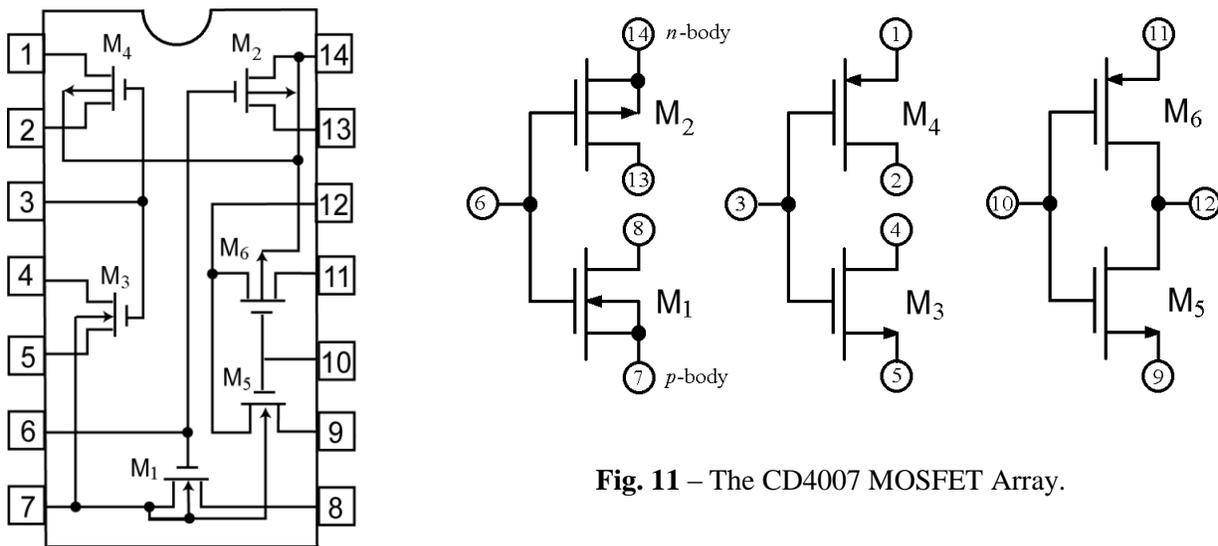
**Fig. 11** – The CD4007 MOSFET Array.
