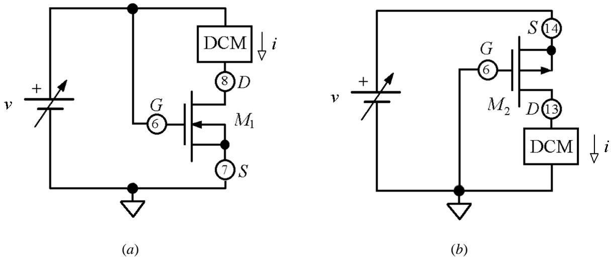
**Fig. 14** – Test circuits to find  $k_n$ ,  $V_m$ ,  $k_p$ , and  $V_{tp}$ .
