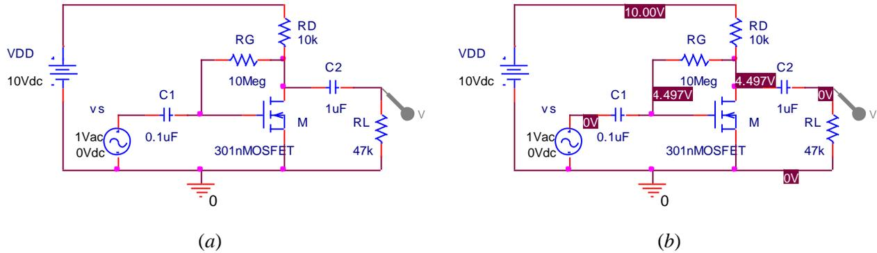
**Fig. 10** – Common-source amplifier and its DC voltages
