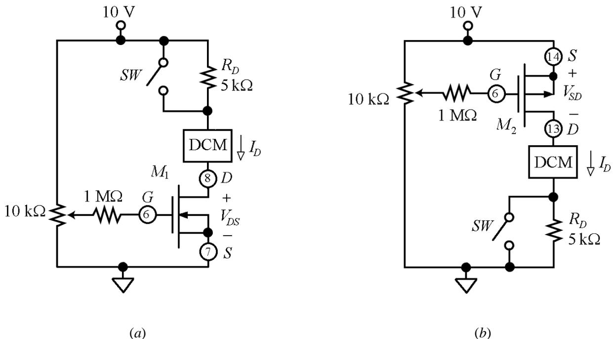
**Fig. 12** – Test circuits to find  $\lambda_n$  and  $\lambda_p$ .
