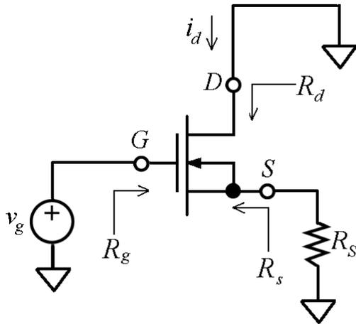
**Fig. 9** – Generalized AC equivalent.
