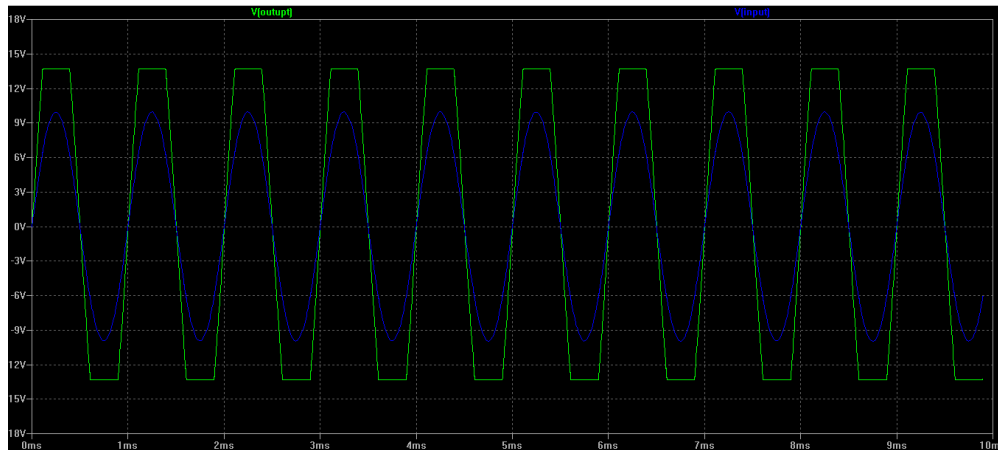
Fig. 11 Clip off The Peak of Output Signal (Green Line)
