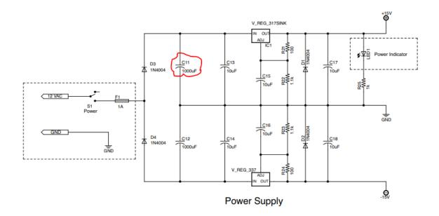
3. Go to your excel sheet part# and search for a cap with 1000uf. Note that this capacitor has a polarity.
